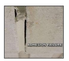
the sealant separates from the substrate. "Failure of cohesion"
